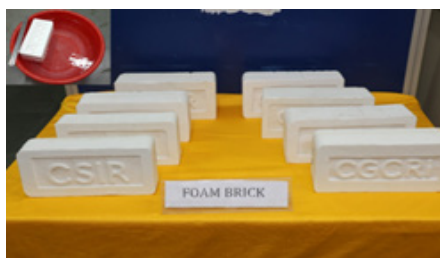
Fig. 1 : Glass foam bricks of dimension 235x110x70 (mm) [Inset: Floating Glass foam Bricks]
